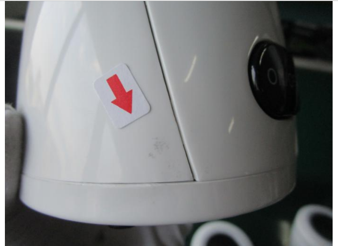
Pic.8 Dirt mark
