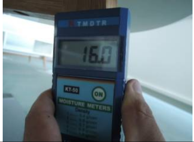
Pic.B Moisture content test was a failed
