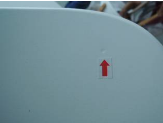
Pic.5 Surface is dent
