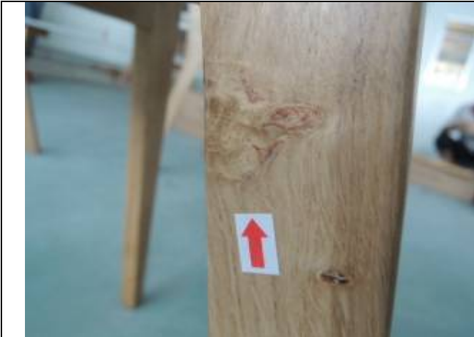
Pic.G Model 9513 legs there are have wooden scar is more than AQL
