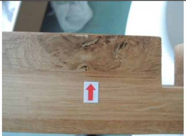
Pic.H Model 9513 legs there are have wooden scar is more than AQL
