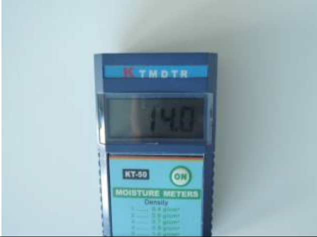
Pic.A Moisture content test was a failed
