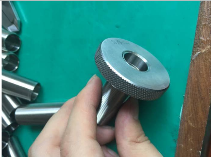
Pic.7 Thread test failed
