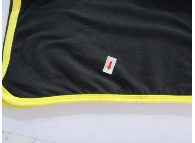
Pic.4 Wrinkled mark at bottom hem.
