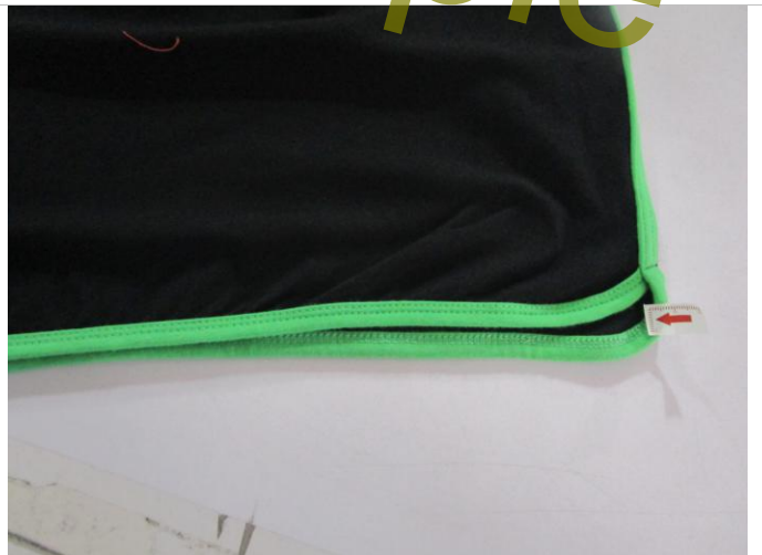
Pic.14 Yellow line not at same level.
