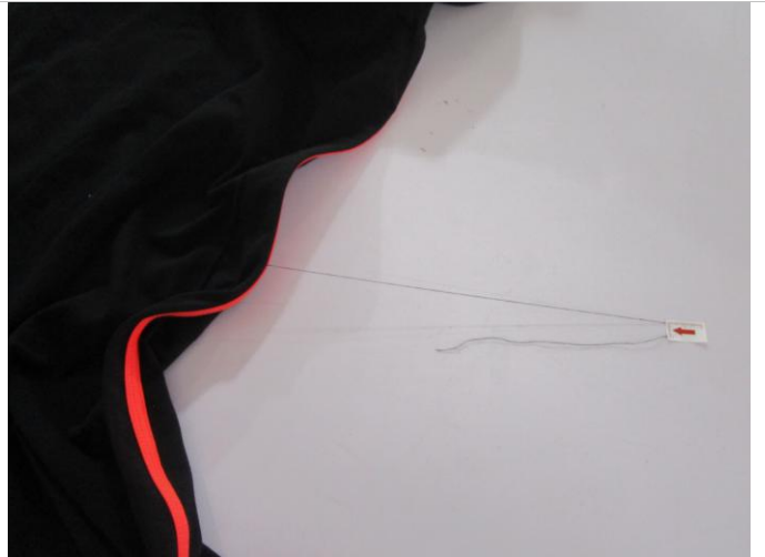
Pic.10 Untrimmed thread ends at seam.
