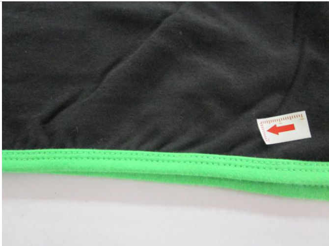
Pic.7 Wrinkled mark at bottom hem.
