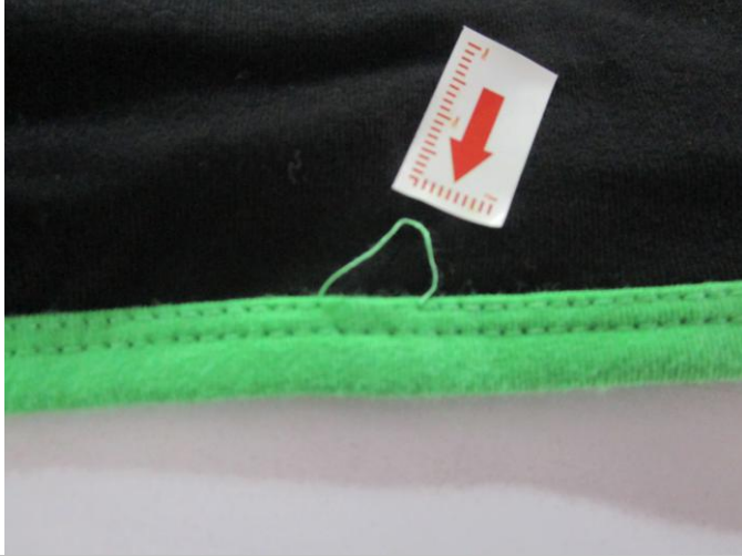
Pic.3 Broken stitching at seam.
